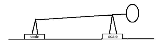
Carry out the experiment. Measure your weight, the force of the floor on your hands, the force of the floor on your feet and any relevant distances. Use the fact that you are in equilibrium and the net force and the net torque must be zero, draw a force diagram for the situation and calculate the location of your center of gravity. Show your work.
