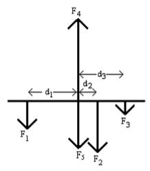
where  $F_1$  is force of the 0.5 kg mass on the rod,  $F_2$  is the force of the 1.0kg mass on the rod,  $F_3$  is the force of the 0.01kg mass on the rod,  $F_4$  is the upward force of the pivot on the rod and  $F_5$  is the mass of the rod.  $d_1$ ,  $d_2$  and  $d_3$  are the distances of the masses from the pivot. Forces  $F_4$  and  $F_5$  are at the pivot.
