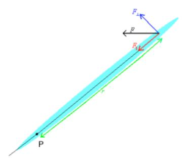
**Exploration 2.1** Do both  $F_{\perp}$  and  $F_{\parallel}$  cause the object to rotate about the pivot point? Explain.
